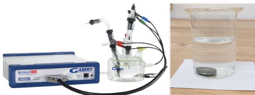
Figure 3. Electrochemical test setup with Gamry Interface 1010E potentiostat and Gravimetric setup with 316L steel samples immersed in 3.5 wt.% NaCl solution.
